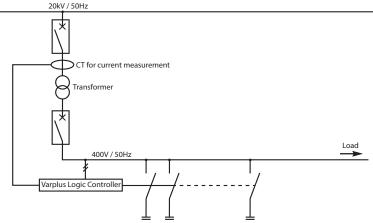
By the current measurement on medium voltage side, the reactive power caused by transformer is measured and regulated by the connected compensation system.
